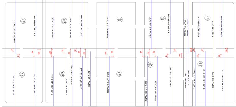
ARMAÇÃO POSITIVA NO EIXO ( Y ) DAS LAJES (0.0)
